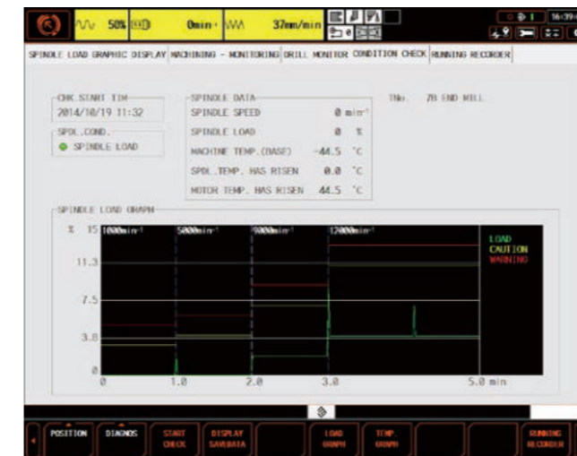
▲ Condition check Temperature as well as the motor load can be displayed.
