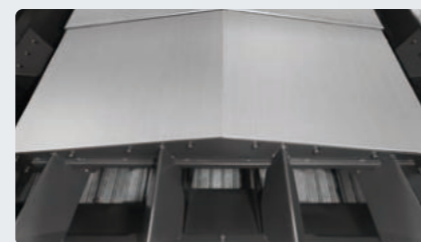
Enlarged chip ducts for smooth chip disposal
