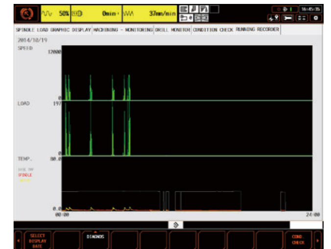
▲ Running recorder Operation status of milling spindle (rpm / motor load) can be recorded for up to one year.
