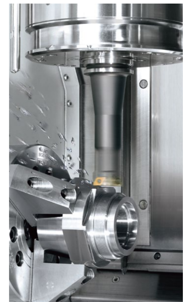
Milling by flash tool
