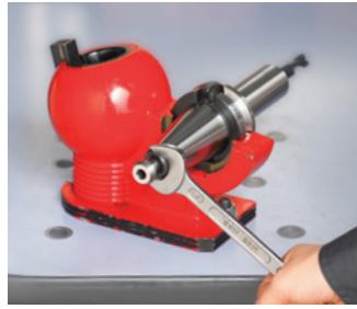
Retention knob tightening
