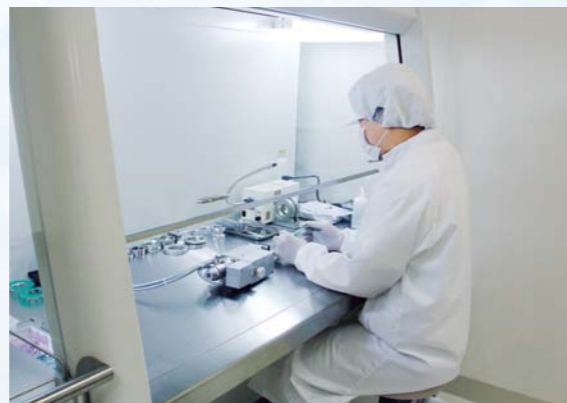
"Clean Bench" used for torch assembly
