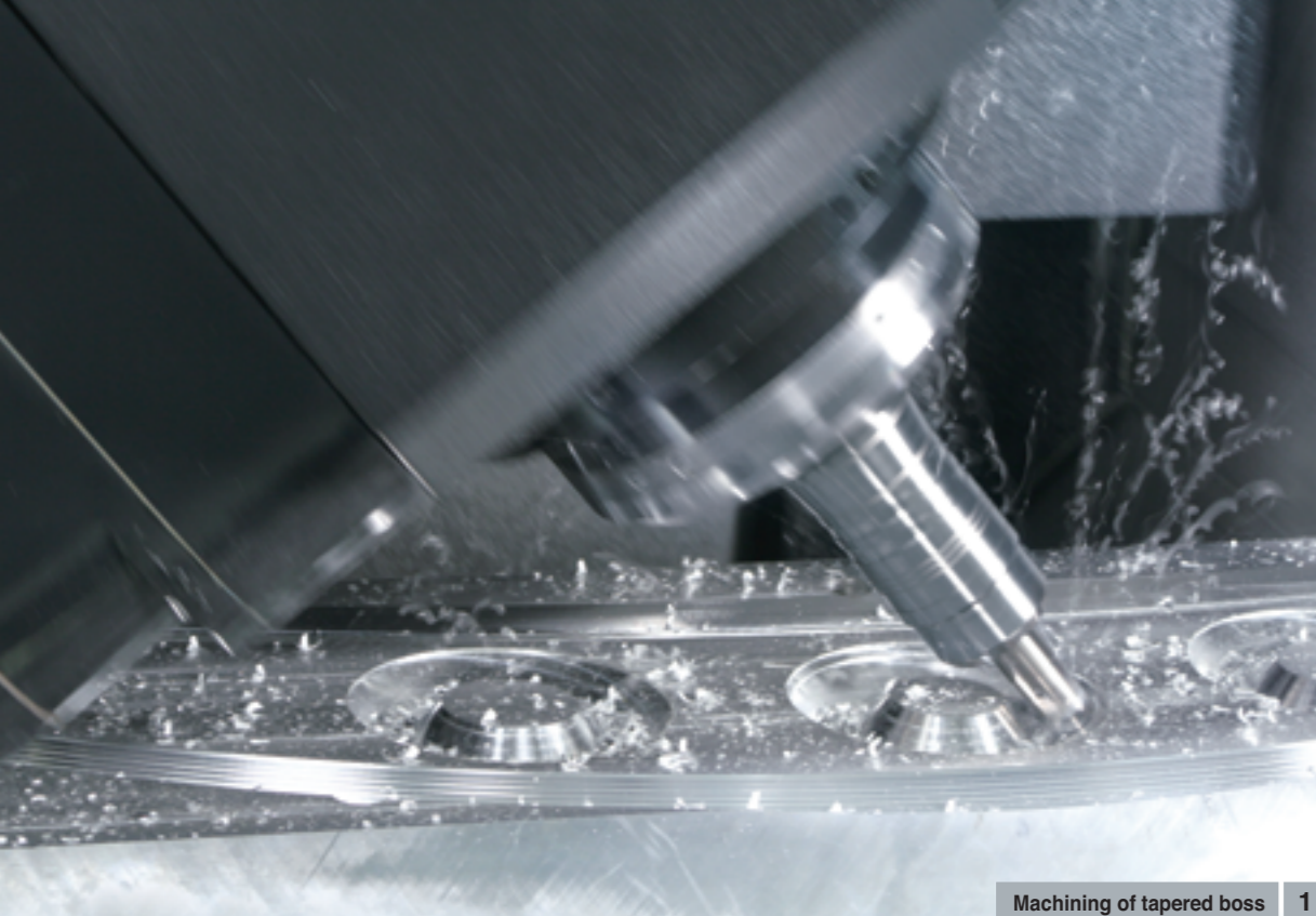
Machining of tapered boss 1
